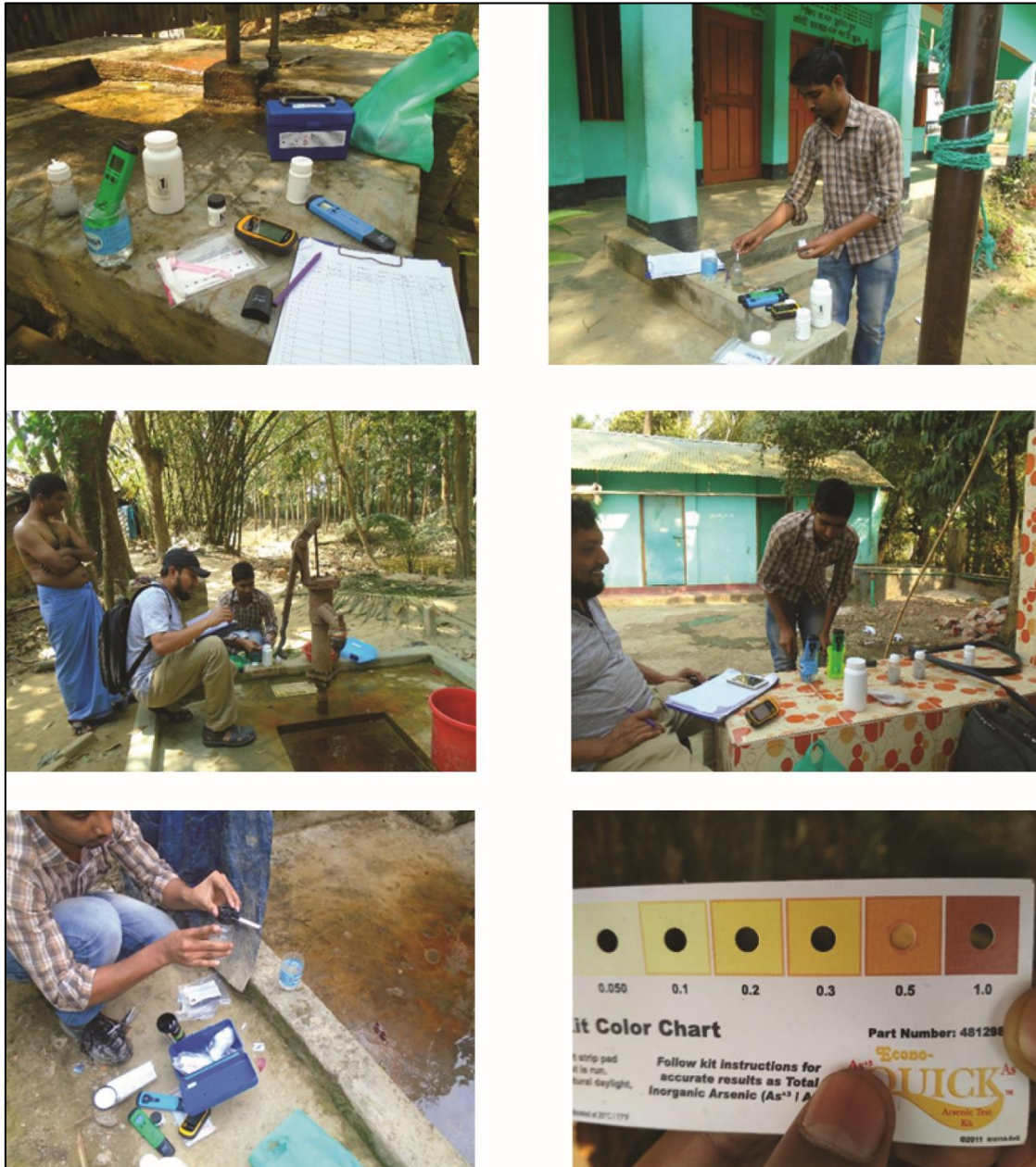
Figure 10: Water Sampling and Field Tests of Arsenic, EC, PH, EH, Temperature etc.
