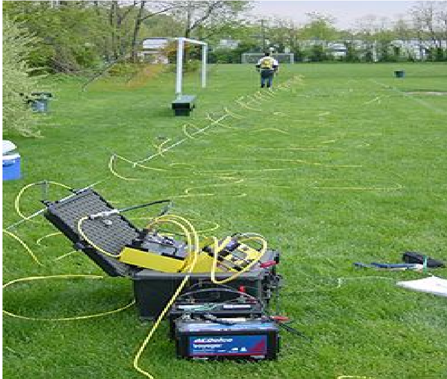
Figure-6: Typical VES setup
