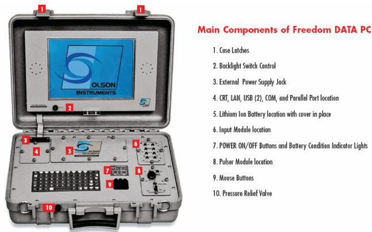
Figure 2.2 Main Component of the Freedom Data PC
