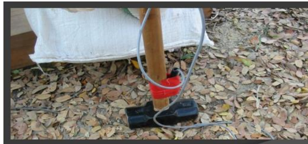
Figure 2.6 To attach the trigger to a hammer.
