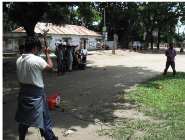
Figure 2.18 MASW Field Data Acquisition
