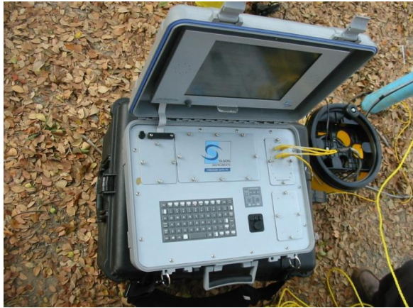
Figure 2.8 To connect the computer with cables which are connected to the geophone.
