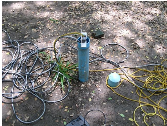
Figure 2.9 Make sure that the air bag at the geophone works. Then, put the geophone into the borehole and fix the safety rope with the holder
