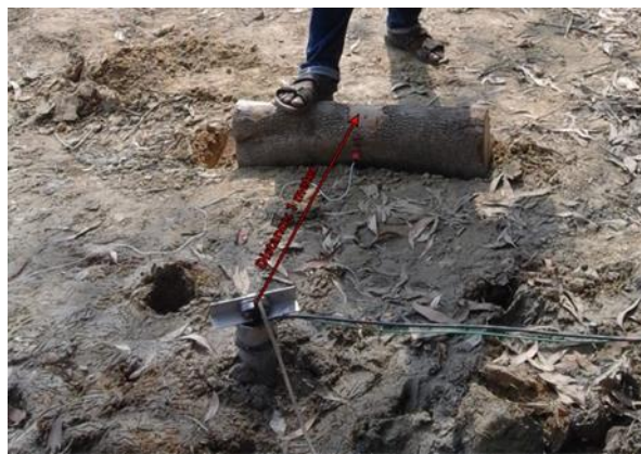
Figure 2.5 To set the wooden plank 1.0 meters from a borehole
