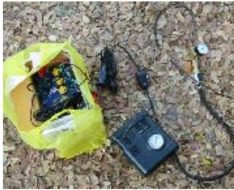
Figure 2.7 To connect the air pump with a battery.
