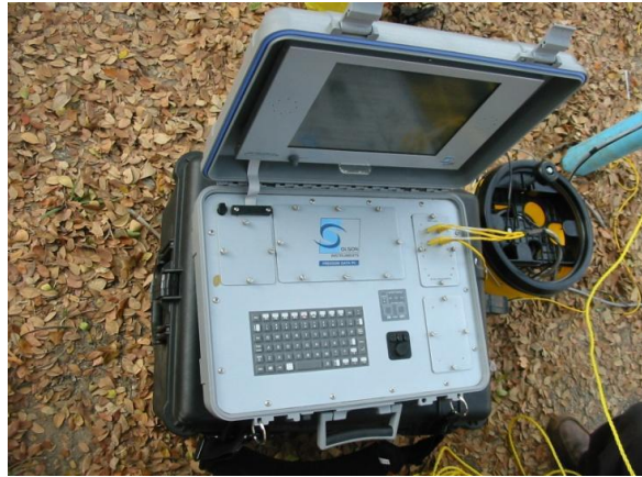
Figure 3.8 To connect the computer with cables which are connected to the geophone.
