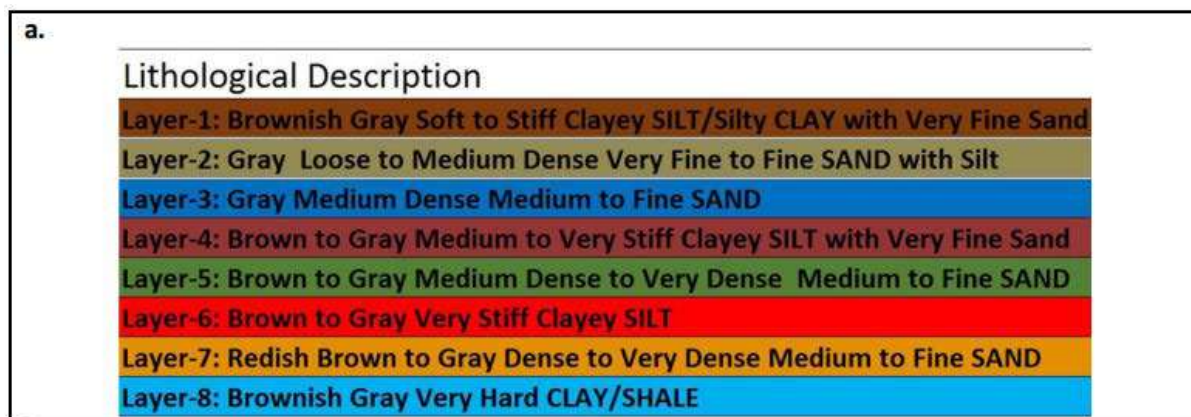
Figure 15. 1: Legend and Lithological Characteristic of Sub-surface of Mirsharai Upazila
